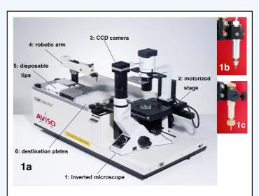
Figure 1: a: Assembly of AVISO's CellCelector<sup>™</sup>, robot for automated cell harvest. b: Scrape tool for harvest of stem cell colonies, c: single cell tool for harvest of stem cell colony fractions
