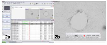
**Figure 2:** Screenshot of the CellCelector<sup>TM</sup>'s control and imaging software. **a:** Picking list and automatically documented snapshots before and after picking of iPSC colonies **b:** stem cell culture on live image with hole where the colony was picked.
